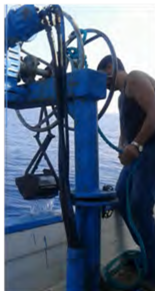
Fig. 2: Sampling process using grab sampler.
